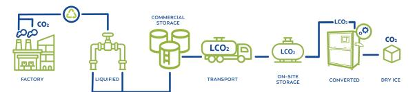
Dry ice is based on the conversion of carbon dioxide ( $CO_2$ ) into a value added, commercially useful product. It's the product of a carbon capture and utilization (CCU) process in which  $CO_2$  is captured from ambient air or at industrial and bio gas facilities, recycled, and converted to dry ice – giving it a second life as a cooling and cleaning medium.
