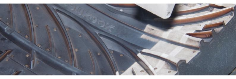
Cold Jet's ASP-T was developed for the automated cleaning of tire molds – inside and outside the press – using the Particle Control System<sup>™</sup> (PCS) with 28 different diamond shaped particles with sizes from 3mm to 0.3mm. The system can be easily integrated into existing processes. This saves up to 70% of the cleaning time compared to conventional cleaning methods.
