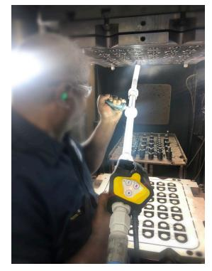
adjustable blast pressure chosen by the user. Stand-off distance and angle of impingement can also have an influence on kinetic energy and, when critical, can be controlled via a programmed robot path.
