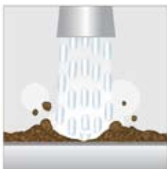
While pellets are most suitable when removing heavy, thick contaminants, shaved ice is ideal for cleaning delicate substrates, intricate geometries or tiny openings.
